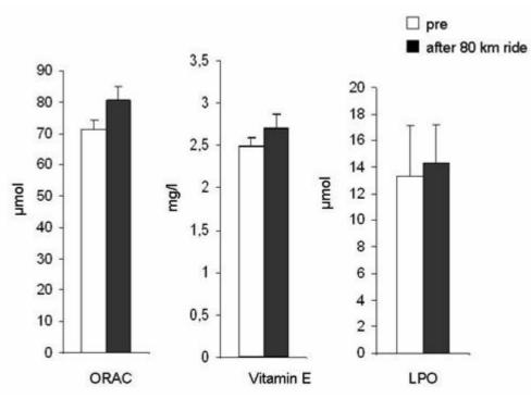
**Figure 1.** Effect of the 80-km ride on plasma ORAC, lipid hydroperoxide (LPO) and vitamin E concentrations in four endurance horses. Values are means  $\pm$  SEM. The level of significance is set at p < 0.05, paired samples t-test.
