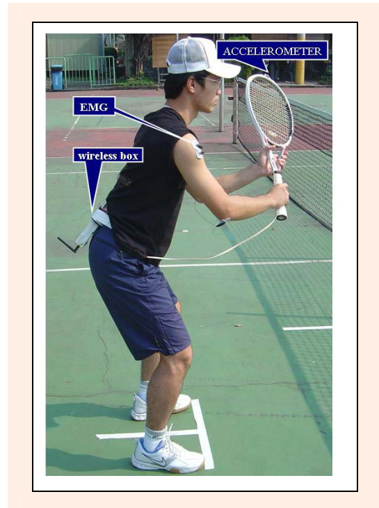
Figure 2. Layout of sensors on the subject: the wireless box is fixed to the back of a participant’s waist, the accelerometer is attached to the top of the racket, and the EMG sensor is taped to the deltoid of the dominant arm.
