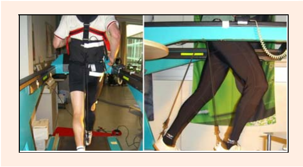
Figure 2. An image of one subject wearing the training device and showing the tube positions.
