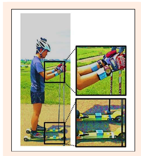
Figure 1. Location of inertial sensors on wrists and roller skis.
