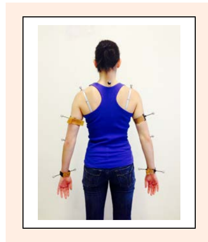
Figure 3. 11 reflective passive markers positioned on the ice dancer anatomical landmarks for the elbow motion analysis.
