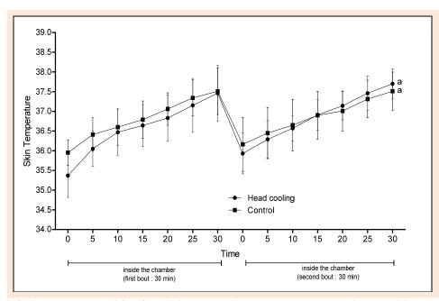
Figure 4. Skin temperature (°C) of participants during the control and cooling conditions (n = 10). "a" indicates large effect size for both trials over time (CON: d = 3.79 and HC: d = 4.89).
