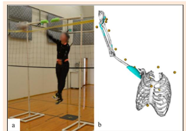
**Figure 1.** a) A subject spikes the ball over the net; prior to ball contact, the ball was resting on the green part of the spike trainer. b) The corresponding MoBL-ARMS model for analyzing the subject's Inverse Kinematics results using OpenSim.
