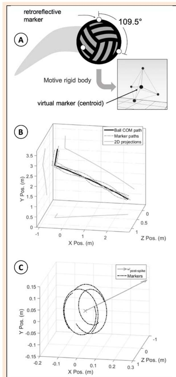
**Figure 2.** a) A ball with tetrahedral markers can be tracked as a rigid body, with a virtual centroid marker. b) In the  $\langle XYZ \rangle$  frame the COM follows a rigid body projectile path in 3D space while the surface markers rotate about the centroid. c) When the path of the markers is considered in the  $\langle xyz \rangle$  frame they trace circular paths with an angular velocity described by the vector.
