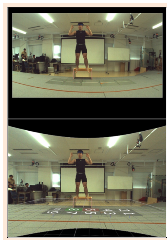
Figure 2. Lens distortion correction by VICON Nexus version of 2.10, using calibration information from the VICON system. Upper figure: pre-correction, lower figure: post-correction.
